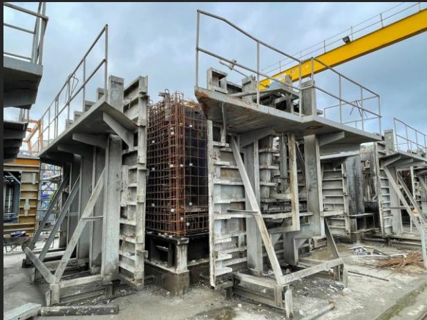
Unique Fixed Moulds for different modules
